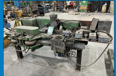
Custom-Built Heavy-Duty U-Shape Rollforming Machine
